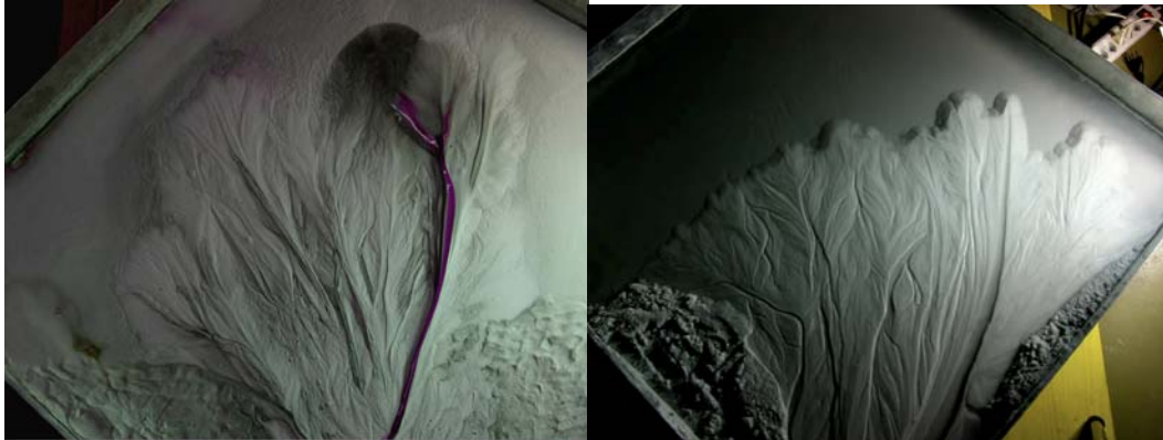
Figure 5 – Comparison between laboratory deltas formed during flow of grains suspended in water terminating in a dry surface (left) and in a liquid ‘sea’ (right). Note that the sedimented layer tapers out continuously in the dry delta case, but drops off abruptly in the wet delta. Other morphological differences are also evident, for example channels tend to be straighter in the dry deltas than in the wet deltas, and more viable channels are present in the wet deltas than in the dry deltas. In the experiment to the left, the flat supporting surface is heated from below to facilitate evaporation (as would occur in the desert), and the inflow of suspended grains occurs in a pulsatile manner (to simulate seasonal storms). The inflow is colored red in the snapshot to the left. In the experiment to the right, grains suspended in water flow continually; experiments using pulsatile inflow here are underway, as are comparisons with cellular automata simulations.
