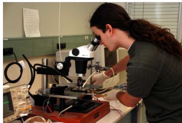
Fig. 3: Colin Boyle uses electrophoresis to orient nanowires
