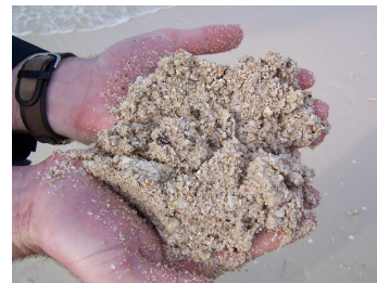
Figure 2. Photo of calcareous sand being used in the land reclamation projects in the UAE.
