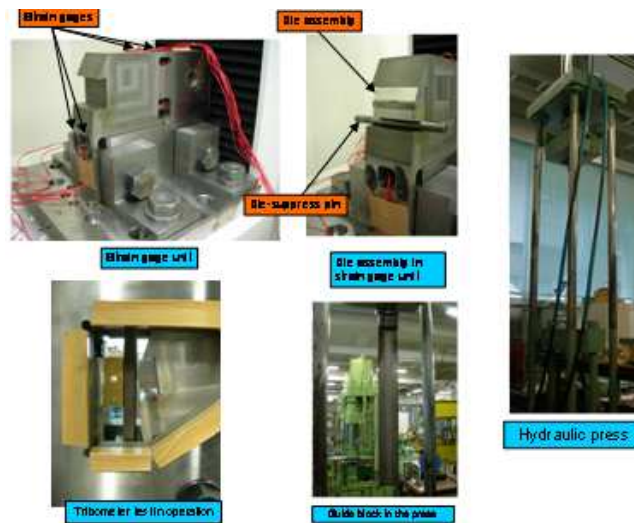
Figure 1. Strip-type ironing test apparatus
